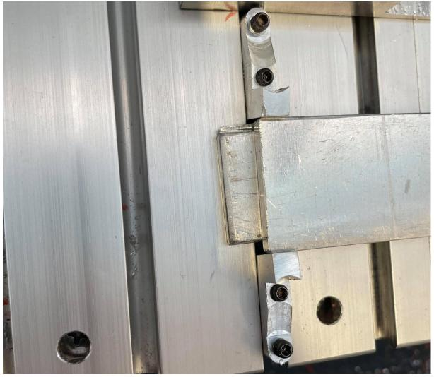
You then need to tighten all the screws, beginning by the #1 screws then the #2 screws. Check if the plate is moving, if it is, you need to tighten it again. Gently hit it with a mallet to put it flat with the surface bellow.
