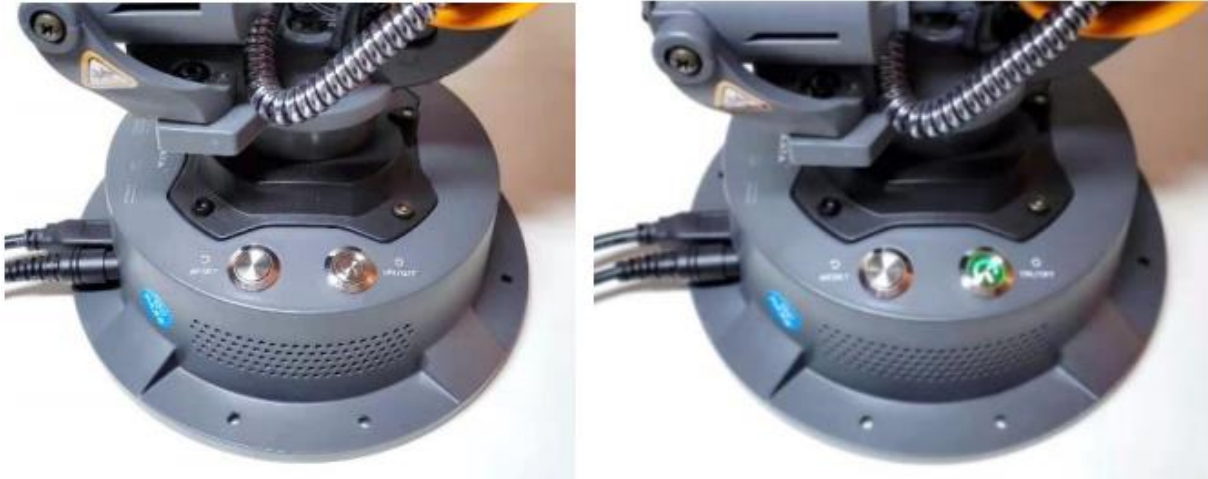
Switching on the manipulator
